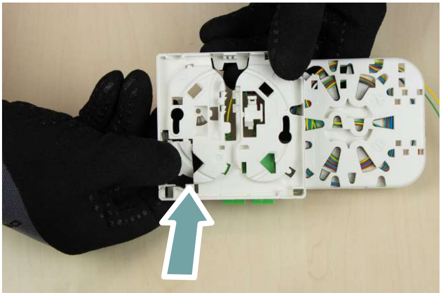
Remove the two breakable plastic parts.
