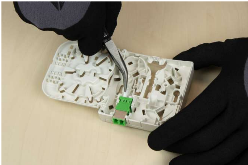
Open the OTO: press the top part of the outlet and remove the lid.
