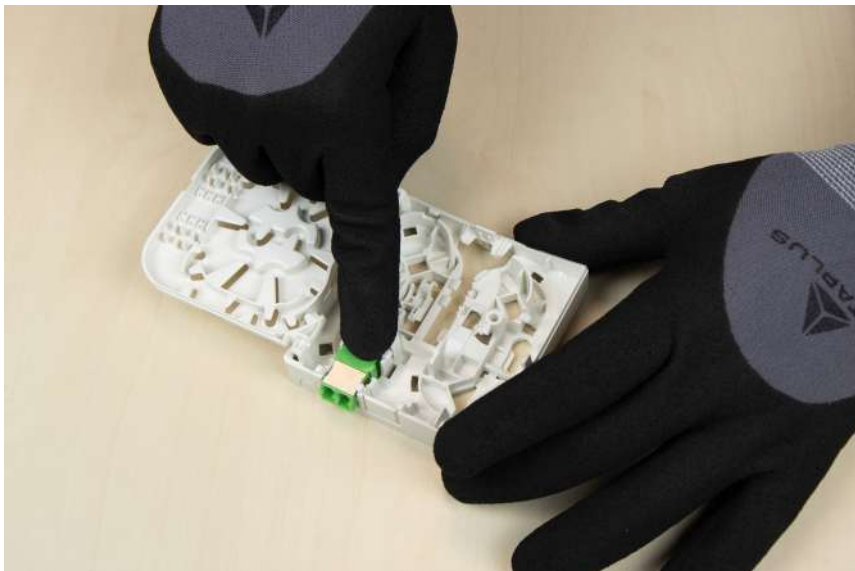
Insert the adapter(s) and clip it(them). Remove the dust caps.
