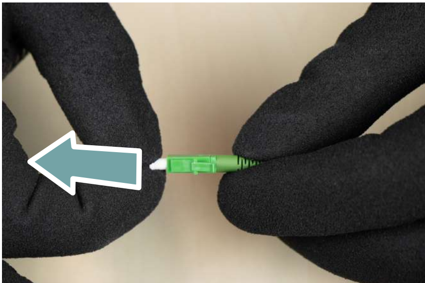
Remove the pigtails dust caps.
